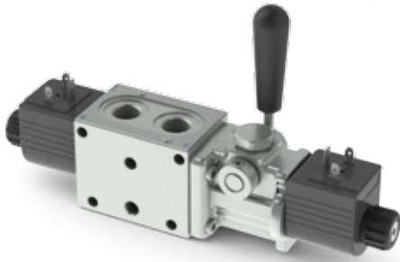
Thanks to his flexibility, the component is designed to be inserted between the valve body and the spool, providing total interchangeability between the different types of solenoid body valves manufactured by Dana Brevini. The control can be used as an emergency device in the event of power cuts.
