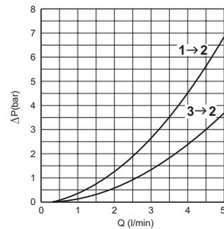
Fluid used: mineral based oil with viscosity 46 mm<sup>2</sup>/s at 40°C.
