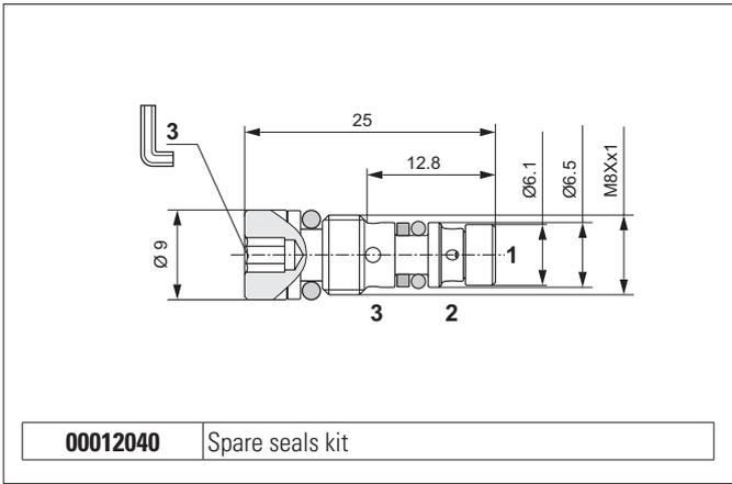
The shuttle type cartridge valves allow taking of the highest pressure signal to the external port via displacement of tempered and ground steel ball. There are usually employed to signal the actuator load to a load sensing pump pressure compensator. External steel body.
