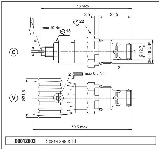
Flow control valve using non compensated throttling. The flow is reduced in both directions, turning the screw or wheel right or left. Guarantees excellent mechanical seal with negligible leakage. It has a galvanised steel body.
