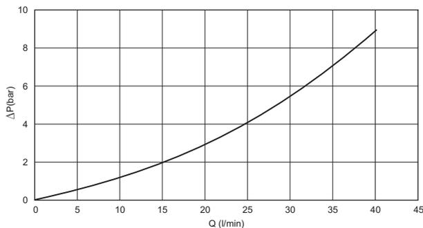
Fluid used: mineral based oil with viscosity 15 mm<sup>2</sup>/s at 40°C.
