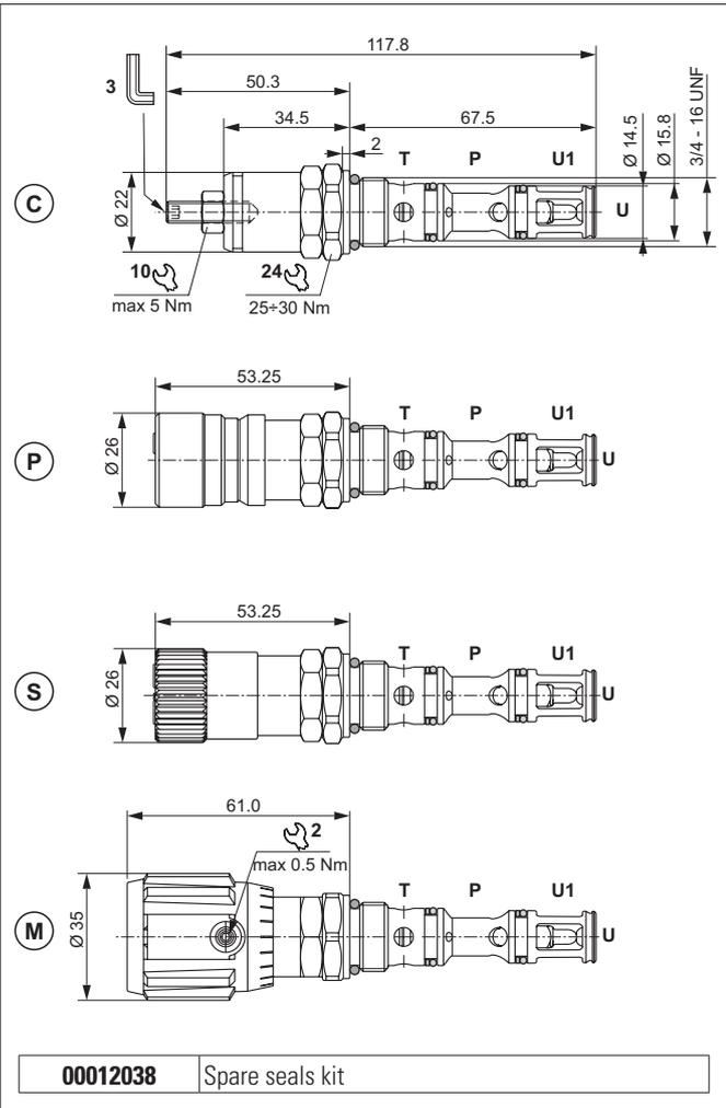
The valve has a combined function in a single cartridge. It consists of a direct acting maximum pressure valve and a unidirectional check valve. The relief valve raises the safety level by making it impossible for the plant operators to set a higher pressure rating, than that specified in the catalogue. It has a pack spring with a mechanical stop.
