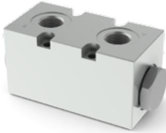
CM3P type modular check bankable valves allow one way free flow by raising a conical shutter, while in the opposite direction the fluid can return by means of a small piston piloted by the pressure in the other line.
