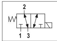
The electric valve is a 3-way 2-position directional electrically controlled valve. Slight leakage is tolerated for this type of valve. The valves work with DC coils whereas RAC coils with a connector with incorporated rectifier must be used for AC applications. The sleeve is in galvanised steel. The plunger is in tempered and ground steel.
