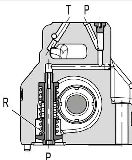
• For the spools 02-04-14-28 the piloting is normally external; the internal piloting is possible with the internal check valve (R).
