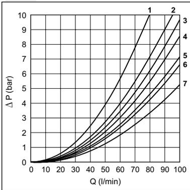
The diagram on the side shows the pressure drops in relation to spools adopted for normal usage (see table).
